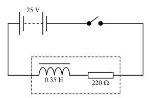
In the circuit shown above, the inductor has inductance 0.35 H and has internal resistance of 220  $\Omega$ . The switch is closed, and after a time of  $8.0 \times 10^{-3}$  s, the circuit current has reached a value that is sufficiently close to the steady current value for any difference to be ignored.
